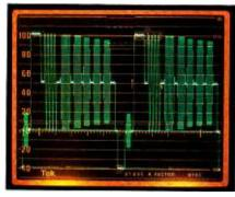
Figure 10. Multiburst signal exhibiting high-frequency rolloff.
