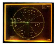
Figure 14. Differential gain of 10% on a vectorscope.
