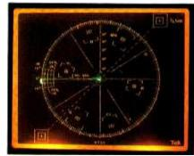
**Figure 12.** Differential phase of 5° on vectorscope.
