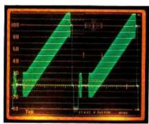
Figure 11. A 100IRE modulated ramp, 2H sweep.
